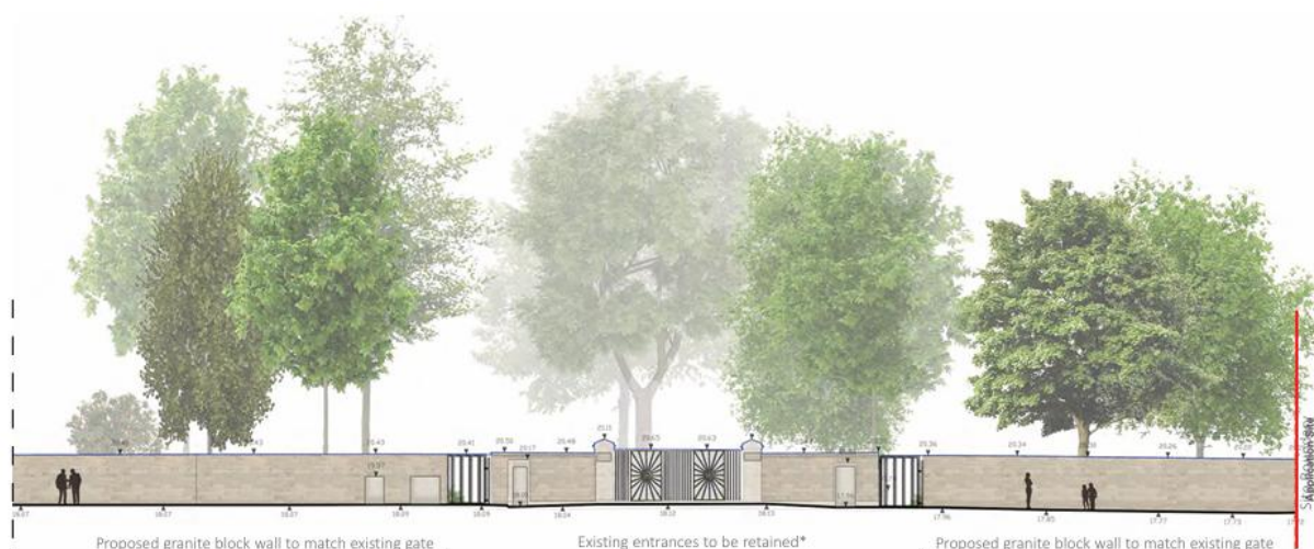
Figure 7.5.10: Existing stone boundary wall treatment onto Sandford Road, as extracted from Cameo & Partners report- denoting the creation of two new pedestrian openings either side of the original gated entrance, page 44 of Landscape Design and Access Statement
