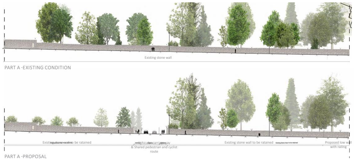
Figure 7.5.7: Existing stone boundary wall treatment onto Milltown Road, (Cameo & Partners)- denoting where a new vehicular opening is proposed, page 41 of Landscape Design and Access Statement
